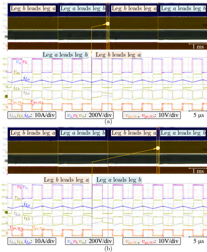
Fig. 19. Experimental waveforms with the gate signal swapping scheme for the two QCM-paralleled GaN HEMT HB legs. The output power P_o = 1.95 kW. (a) Transition from HB leg a leading leg b to leg b leading leg a ; (b) transition from HB leg b leading leg a to leg a leading leg b .
